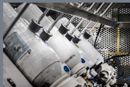
The size of each cylinder may vary due to flexible connections and a pneumatic and automatic safety fixation.
