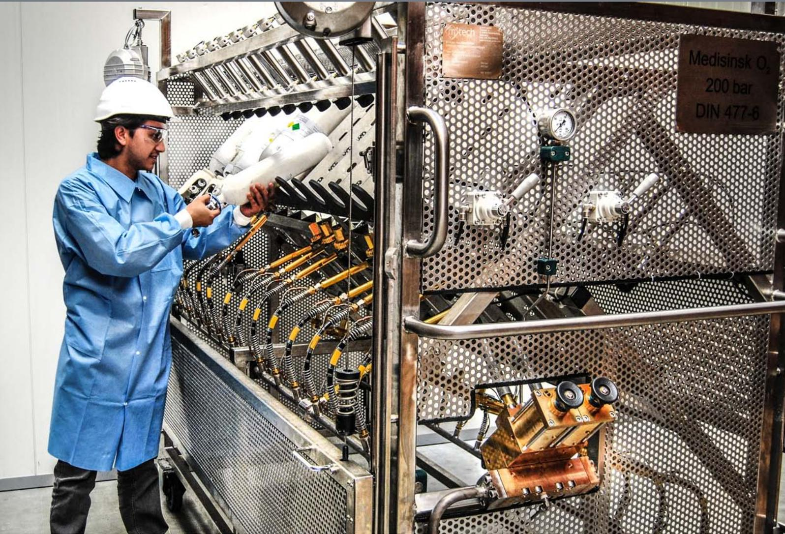
m-tech gmbh has realized a solution which increases the flexibility of its customers, changing from a fixed installed filling station to a complete and moveable filling trolley that meets all standards in safety.
