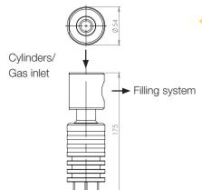
Particulate traps can prevent penetration of particles into the filling system
