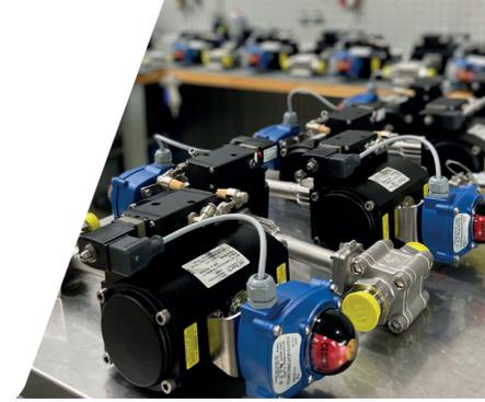
m-tech's ball valves are specially designed and manufactured to meet relevant cryogenic standards (DIN EN 1626, BS 6364). The valve are suitable for handling cryogenic liquefied gases such LIN, LAR, LOX and LNG.
