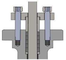
In order to perform the replacement of packing, the valve should be properly supported.
