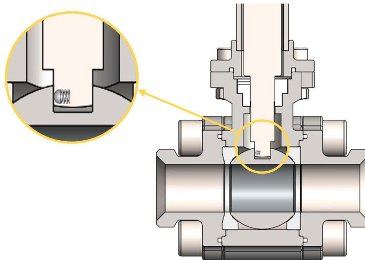
2. A conductive stem seal (Carbon filled PTFE) ensures the contact between the stem and bonnet/body.
