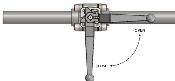
The LCV is in open position, when the hand lever in line with the pipeline is and in closed position, when the handle perpendicular to the pipeline is.
